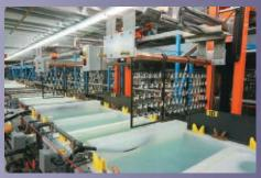
With the completion of our new, state-of-the-art electroplating facility, we can now offer contract plating with the same quality of finish our connectors have long featured. Our fully-automated, robotically controlled line has analytical measuring hardware and software at each stage for real-time monitoring and adjustment of plating parameters.
