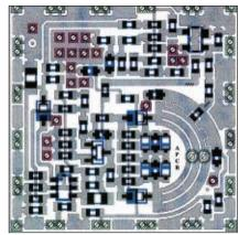
Fig. 14 Typical layout of a 12 GHz MC VCO active planar coupled resonator (APCR).
