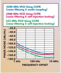
Fig. 9 Measured phase noise for a CCPR VCO.
