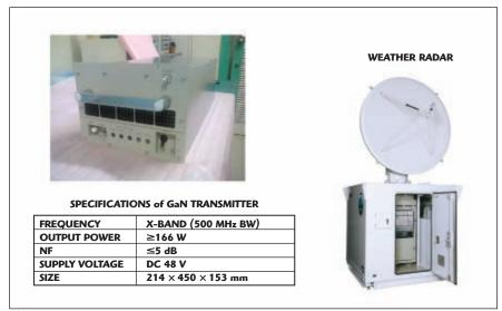
📤 Fig. 15 Weather radar with GaN SSPA transmitter.
